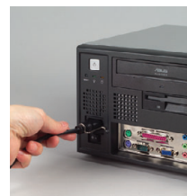
Plug ring-lock securely fastens the power cord
